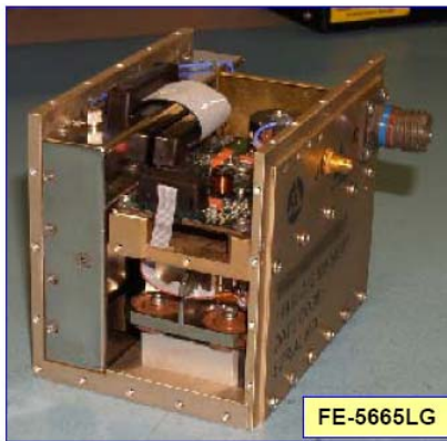
Figure 8. G-Compensated quartz oscillator integrated with rubidium atomic standard
