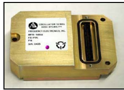
Figure 5. Hard mounted stand-alone g-compensated multiple-output frequency generator unit (Size L x W x H inches 3.7 x 2.5 x 1)
