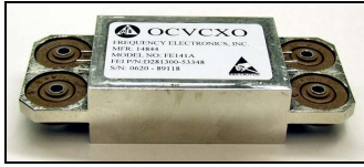
Figure 6. "Soft" mounted stand-alone g-compensate oscillator (Size L x W x H inches 4 x 1.6 x 0.8)
